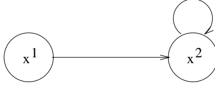
Figure 3.3: A two-states Markov chain for which a least-squares approximation method for cost calculation may diverge.
