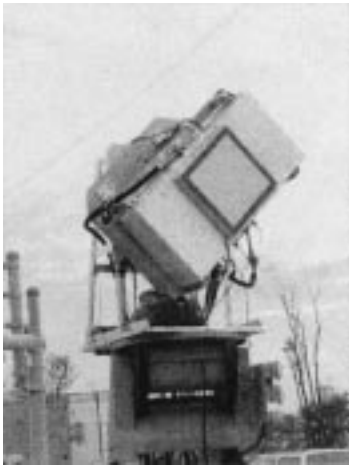
Fig. 10. EA phased-array antenna assembly.
